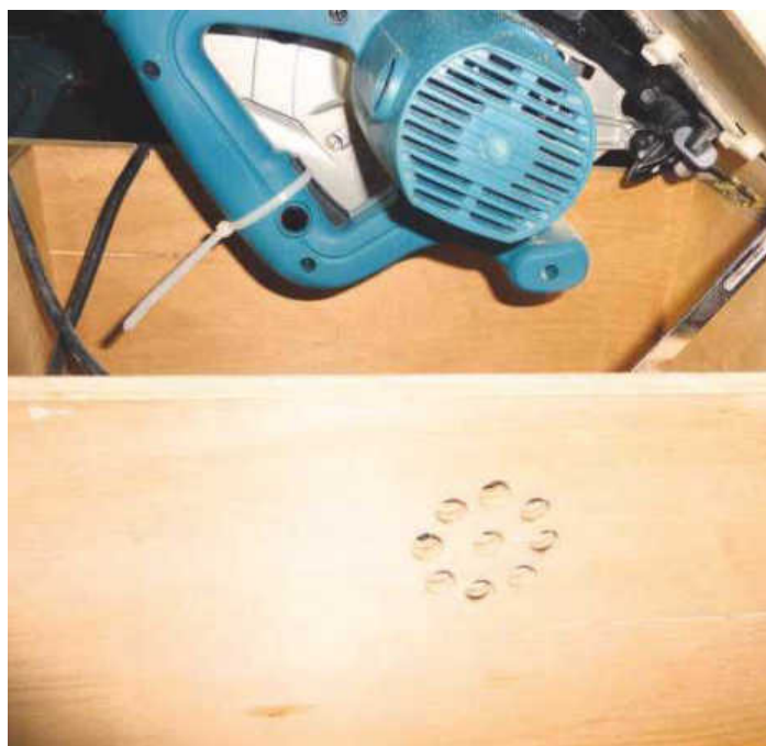
PIC 4. An array of breathing holes allow the motor to suck in fresh air
